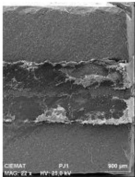
Figure 4: SEM image of cross-section Brazil module.
