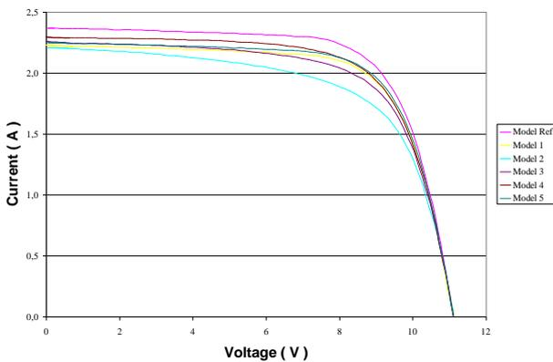
Fig. 1: The (I-V) curves of clean modules measured after long-term outdoor exposure.
