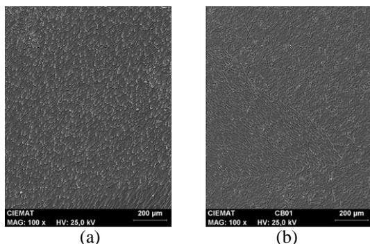
Figure 5: SEM image of SiO<sub>2</sub> films. (a) Brazil module and (b).
