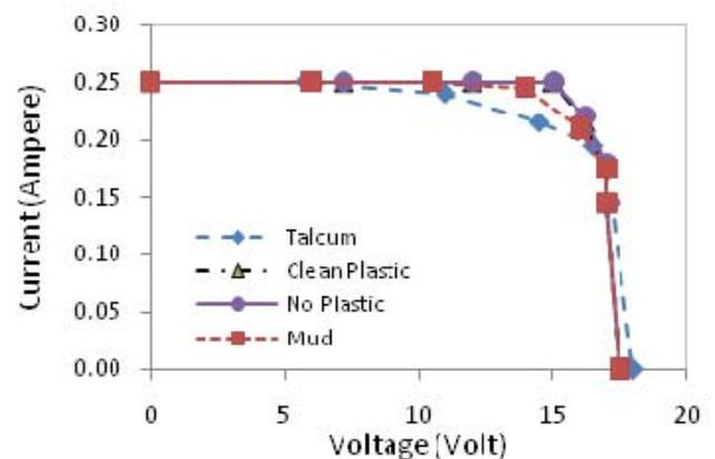
Fig. 8 *I-V* characteristics for irradiation of 301 W/m<sup>2</sup>
