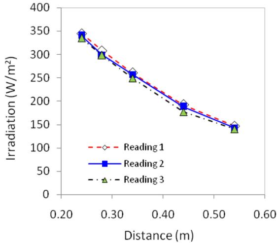
Fig. 6 Irradiation versus distance for two spotlights
