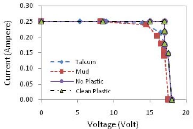
Fig. 7 *I-V* characteristics for irradiation of 255 W/m<sup>2</sup>
