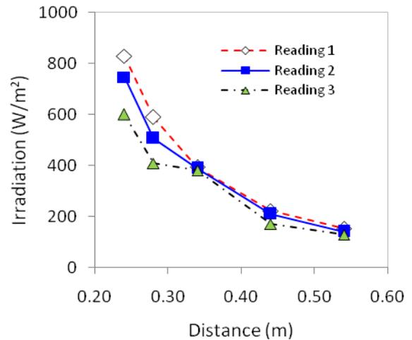
Fig. 5 Irradiation versus distance for one spotlight
