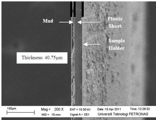
Fig. 3 SEM image for thickness of mud layer
